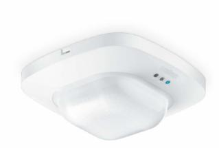
The IR Quattro HD DCS is a digital, high definition, passive infrared presence detector setting a new standard in lighting control with minimal movement required for human presence detection. It features four pyroelectric detectors with a high performance lens system that creates a new global standard in detection with 4,800 switching zones. Included light level feature provides the option to dim and turn lights off when sufficient daylight is present for additional energy savings.
